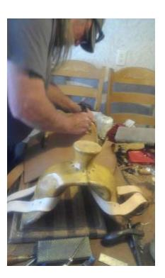
Next we did the back part of the cinch/hangers we stitched it together - again mostly Jim doing the layout and cutting and me driving nails and attached it to the cinch rings using leather laces.
